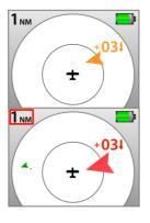
In dangerous situations, aircraft posing a threat are presented in orange or red, depending on the urgency of the threat. An acoustic warning is issued in addition to the optical warning.
